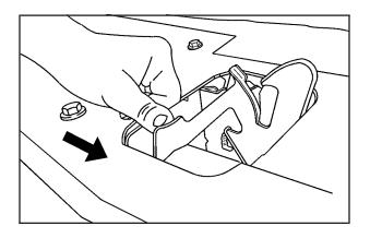
2. Then go to the front of the vehicle and push the secondary hood release handle toward the driver's side of the vehicle.
